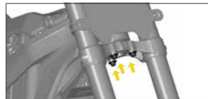
2. After removing, pre-install the T-shaped gaskets on the three bolts respectively, and pay attention to the direction of the T-shaped gaskets as shown in the figure.
