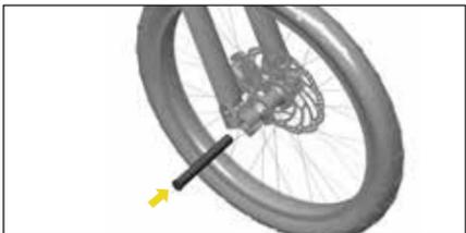
6. Secure the left and right lock nuts with an 8# inner hexagon wrench.
