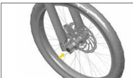
7. Tighten the four bolts at the bottom of the front fork with a 4# inner hexagon wrench.
