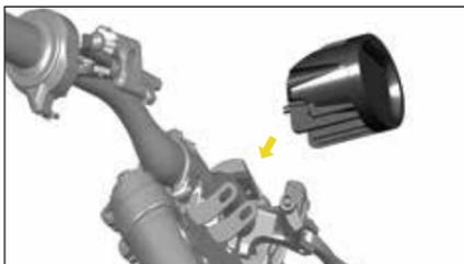
2. Adjust the position and tighten the screws on both sides.
